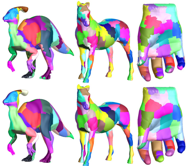
Figure 2: Top row shows initial chart partitions, and bottom row shows result of chart boundary optimization.
